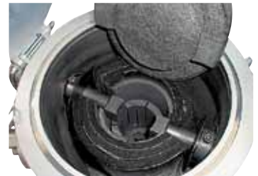
Graphite heating module
