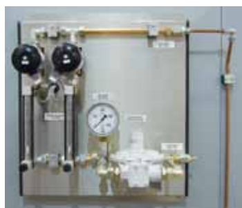
Gas supply system for non-flammable protective or reaction gases
