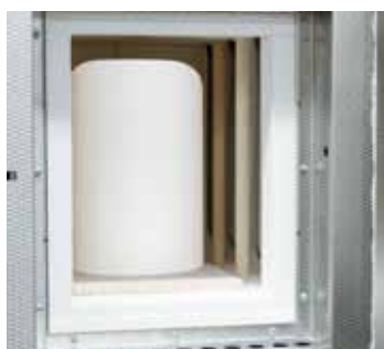
Inner process hood with gas injection through the furnace bottom protects the furnace chamber against contamination and/or prevents chemical interaction between the charge and heating elements
