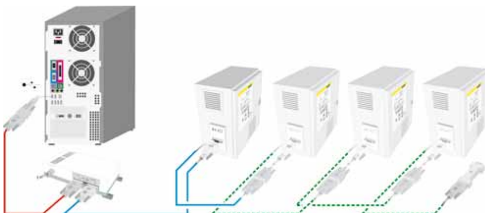
Extendable for connection of up to 16 furnaces
