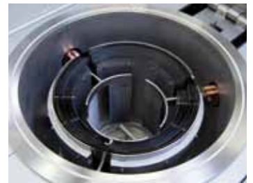
Cylindrical retort with tungsten heating
