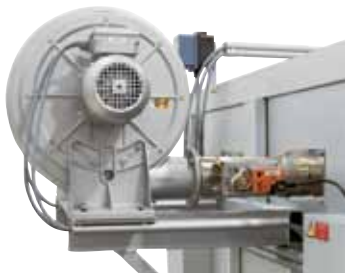
Cooling fan for accelerated cooling
