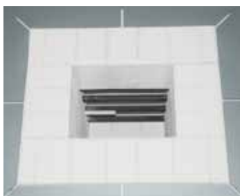
Two-Side heating with SiC rods
