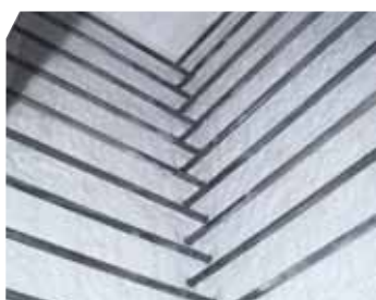
Heating from 4 sides with SiC rods
