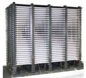
Measurement setup for determination of temperature uniformity in the useful dimensions of the furnace
