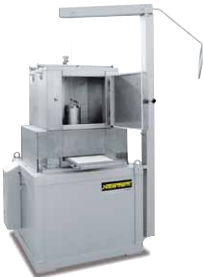
TS 30/18 with preheating chamber above the salt bath and crane to dip the charge in
