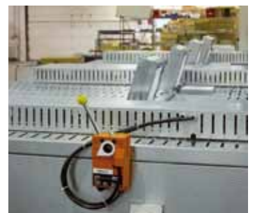
Motor-driven exhaust air flaps as additional equipment
