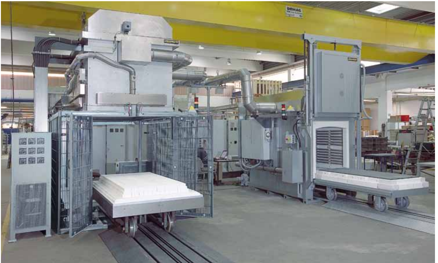
Production system consisting of a bogie hearth furnace for debinding and a high-temperature furnace for residual debinding and sintering with shared catalytic afterburning system
