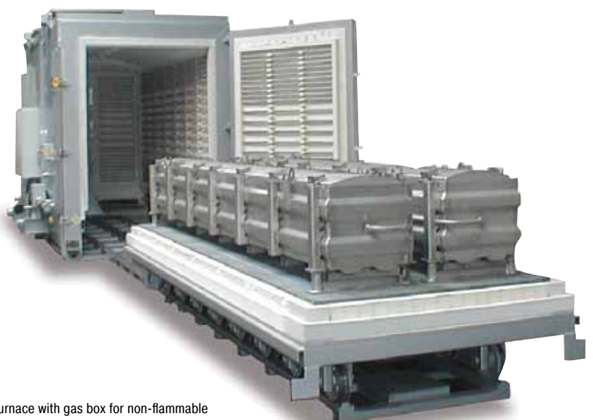
Bogie hearth furnace with gas box for non-flammable protective or reaction gases
